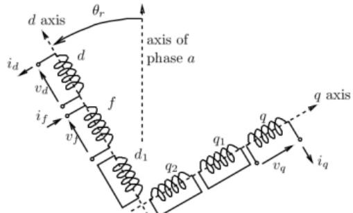
3-phase stator replaced by  $d, q$  windings.
