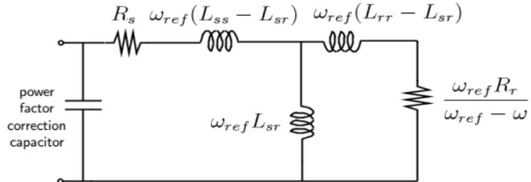
$$\text{Dynamics of rotor speed : } 2H \frac{d\omega}{dt} = T_e - T_{mo}(A\omega^2 + B)$$
