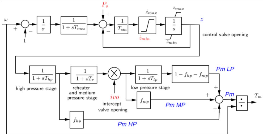
Turbine nominal power  $P_{nom} = 460$  MW. All variables in pu on the  $P_{nom}$  base.
