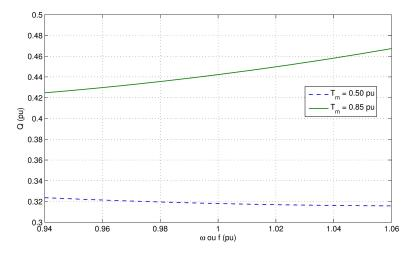
The slope is positive or negative, depending upon the mechanical load !
