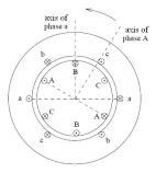
Motor sign convention at both stator and rotor.
