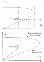
When *z* increases, the load characteristic changes until it eventually does not intersect the network characteristic. Equilibrium is lost at the *loadability limit*.
