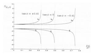
It can also be shown that the sensitivity changes from positive to negative as the operating point moves from the upper to the lower part of a PV curve.
