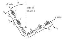
The Park transformation consists of replacing the (a, b, c) stator windings by three equivalent windings (d, q, o):
