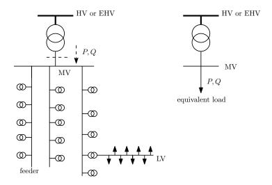
Thanks to its simplicity, the above individual model is frequently used to characterize the power consumed by a set of loads of similar nature
