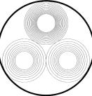
"snapshot" of the equipotential lines when each of the three phase conductors has its own sheath
