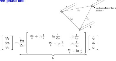
• derived assuming that  $i_a + i_b + i_c = 0$  (no current outside the 3 conductors)
